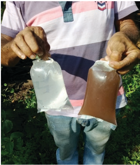
In the picture above, the water sample seen on the left has been collected by Sema technicians for analysis at the collection point of Gusa Nordeste. The water sample seen on the right, has been collected at the disposal point, it is water discarded by the steel mill into the Piquiá River, after the cooling of the blast furnaces. ©ACMP
